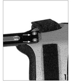
**1.** Pull back the pad on the inside of the lower shell of the Thruster RLF Brace (LA or MA). Apply the AFO Attachment to the outside of the upright, and insert the screws from the kit through the holes. Attach the screws to the threaded holes from the inside of the upright, as indicated in photo, into the extension upright of the AFO attachment.
